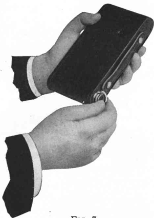
FIG. 7 Turning a new section of film into position
